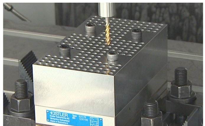
Screw tapping with a Type 9257B dynamometer
