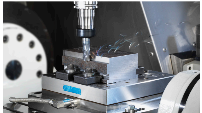
Milling with a Type 9255C dynamometer
