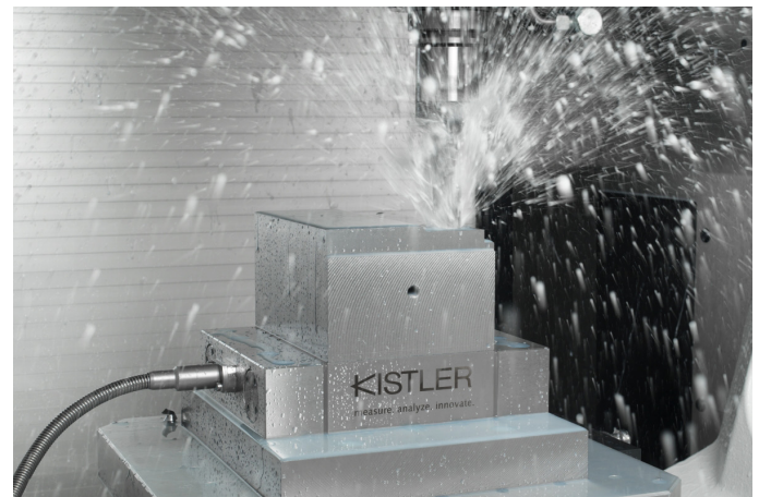
Milling with a Type 9139AA dynamometer
