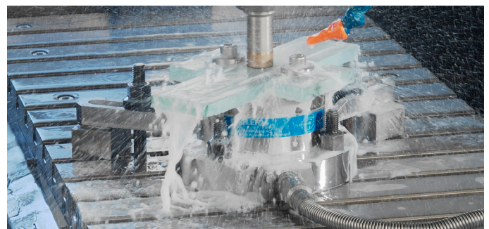
Force measurement during quartz cutting with a Type 9272 dynamometer
