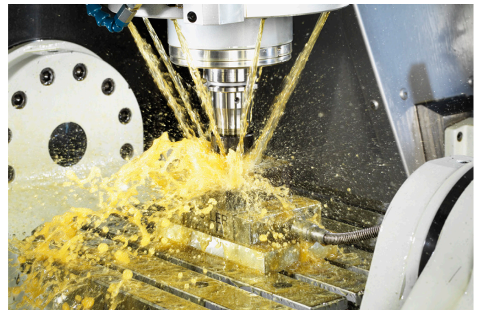
Milling with a Type 9129AA dynamometer
