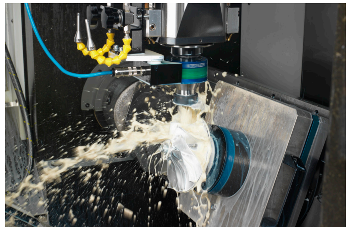
Milling an impeller with a Type 9170A rotating dynamometer
