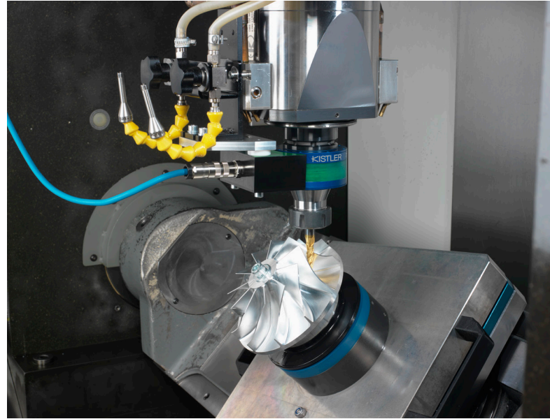
Rotating dynamometer in use during machining of an impeller
